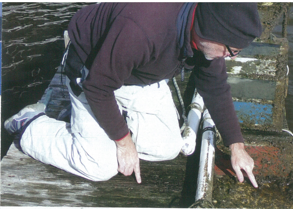
Tech editor Drew Frye checks bottom paint panels after one-year in the brackish waters of Chesapeake Bay.
