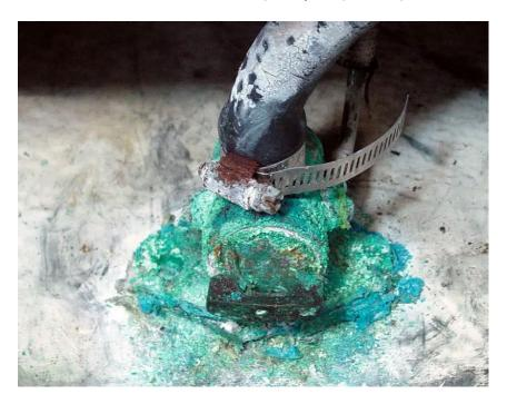
Considering the excitement a failed seacock can generate, the lack of attention they typically receive is almost criminal. Tucked away in the dim recesses of your bilge, seacocks typically don't get a second thought with regards to preventative maintenance or inspections – until they fail to operate or even break off in your hand during operation (it happens, I've seen it, and it isn't pretty).
